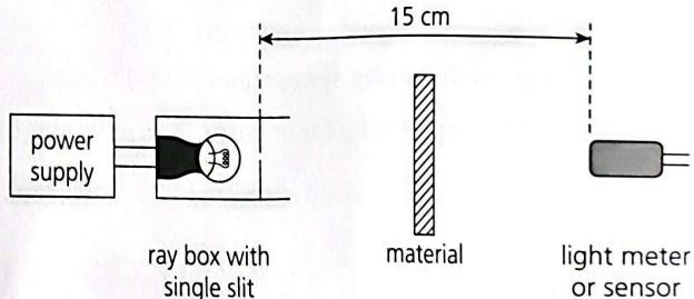
a. Is the meter measuring how much light is transmitted or reflected?
